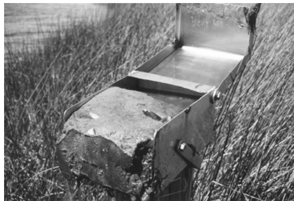
Figure 3. Benthic sampler used by scuba divers to collect fully enclosed sediment samples
