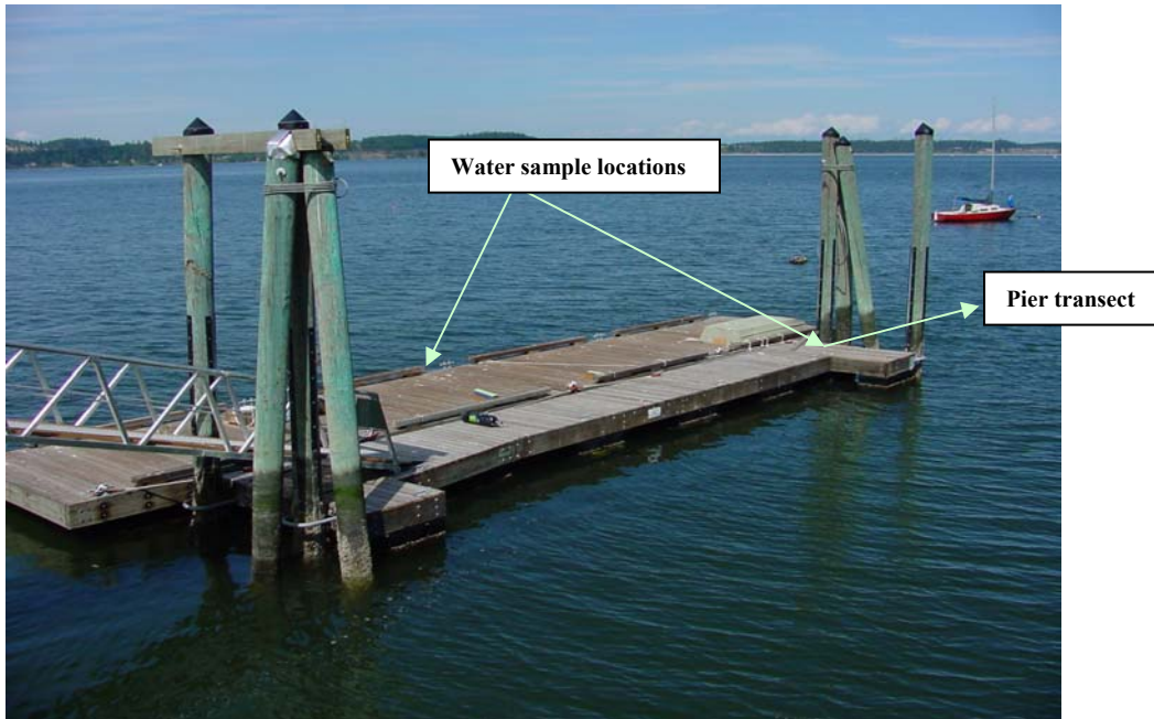
Figure 1. ACZA treated float in Sequim Bay, Washington that was subject of a risk assessment conducted on October 18, 2002. Triplicate water samples were collected at a local reference location and at the indicated locations adjacent to the structure during a rainstorm on December 13, 2002. Water collection depth was 0.1 m along side the float and 0.5 m in the center of the dolphin.
